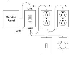
Always place Outlet Branch Circuit Type AFCI in position A. All outlets of the protected branch, including lighting and receptacle oulets must be connected to the load side of the AFCI.
