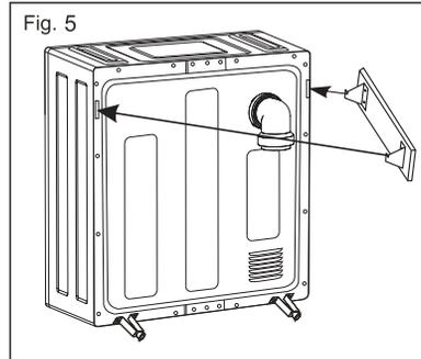
The appliance shall not be exhausted into a chimney, a wall, a ceiling, an attic, a crawl space, or a concealed space of a building.
