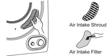
Slightly push upwards with your thumb until the latch hook disconnects, then remove.
