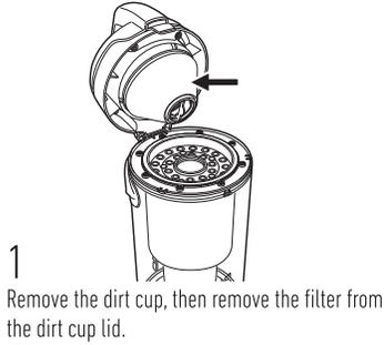
1 Remove the dirt cup, then remove the filter from the dirt cup lid.
