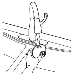
2 Rinse filter with water only until the filter is clean and the water runs through clear. Gently squeeze the filter to remove excess water.
