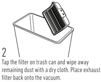
2 Tap the filter on trash can and wipe away remaining dust with a dry cloth. Place exhaust filter back onto the vacuum.
