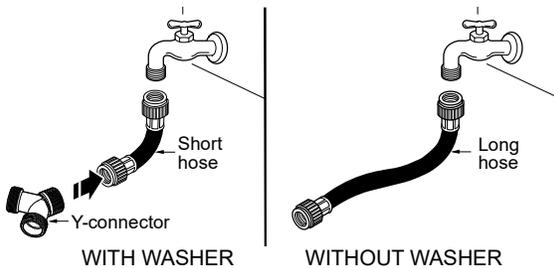
Connect all water supply hoses tightly by hand and then tighten another 2/3 turn with pliers.
