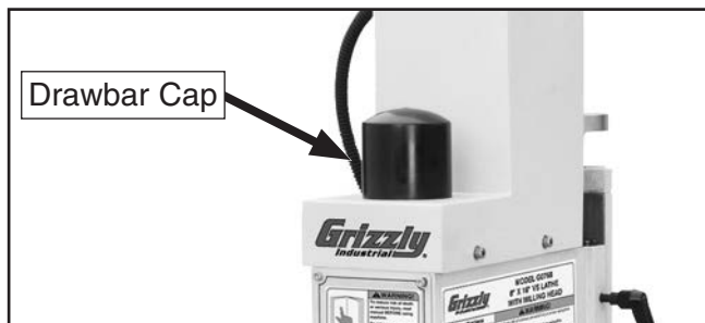
Figure 111. Location of drawbar cap.
