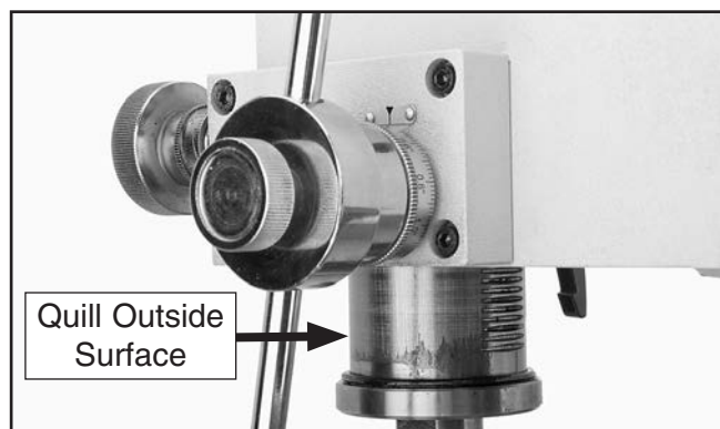
Figure 135. Outside surface of quill.
