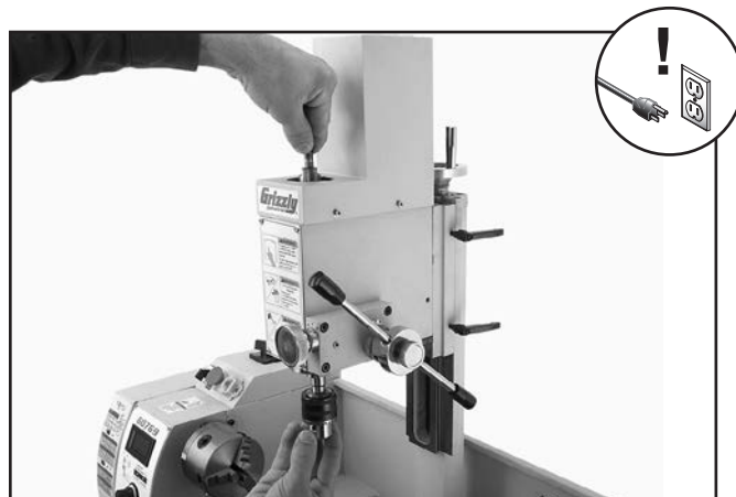
Figure 112. Threading drawbar into tooling.
