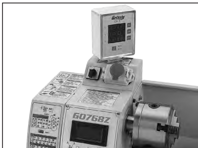
Figure 1. DRO magnetically mounted on lathe headstock.
