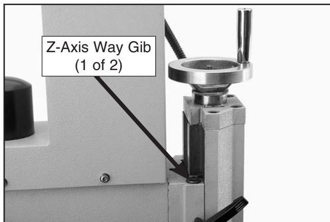
Figure 147. Location of top Z-axis way gib.
