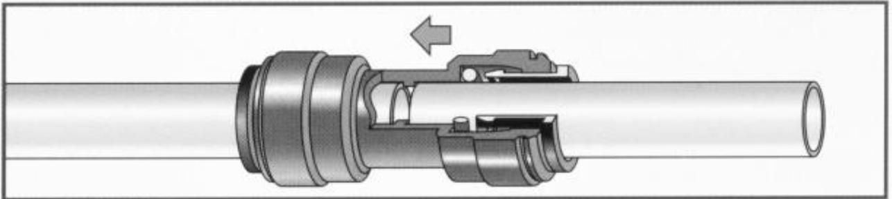
Push the tube into the fitting, to the tube stop. The collet (gripper) has stainless steel teeth which hold the tube firmly in position while the 'O' ring provides a permanent leak proof seal.
