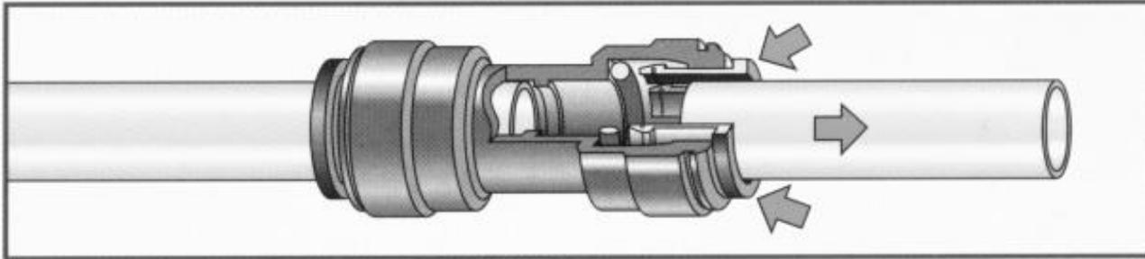
To disconnect, ensure the system is depressurized before removing the tube. Push in collet squarely against face of fitting. With the collet held in this position, the tube can be removed.
