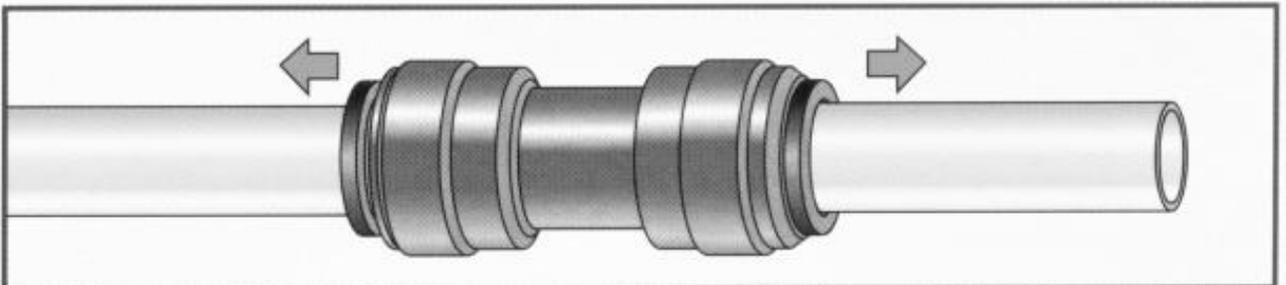
Pull on the tube to check that it is secure. It is a good practice to test the system prior to leaving site and/or before use.
