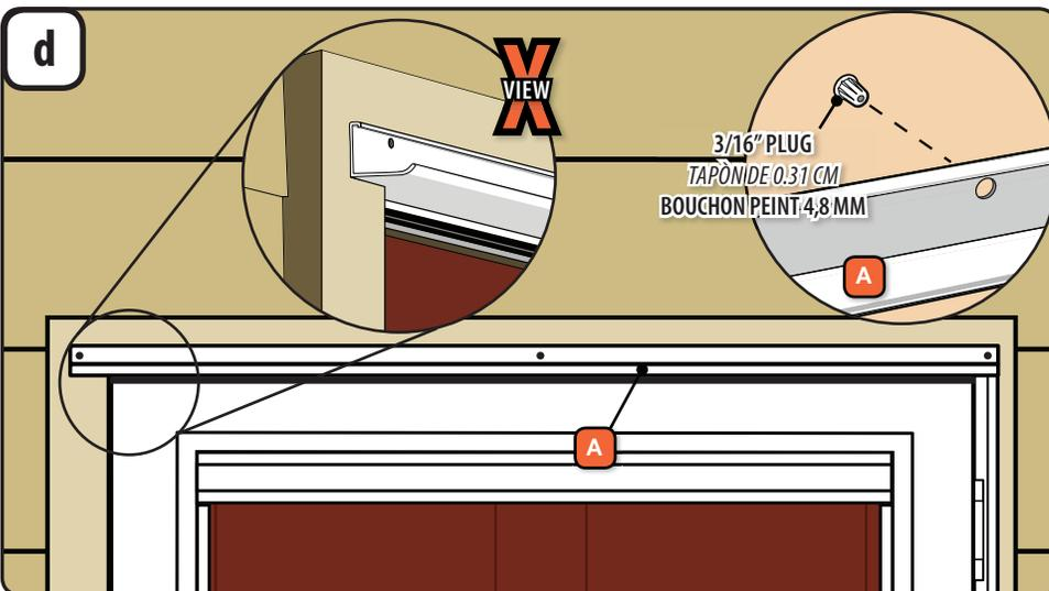
1. Open the storm door. Place the rain cap (A) in the opening so that it rests on top of the hinge rail, aligning the end of the the rain cap with the edge of the hinge rail.
