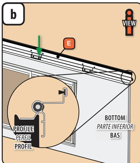
1. Position the hinge rail along the hinge-side edge of the door frame so the bottom hole of the 2nd hinge up from the bottom lines up with the bottom hole from the screw removed in **step 7a**. **NOTE:** The top of the hinge rail should extend approximately 3/16" beyond the top of the door frame.
