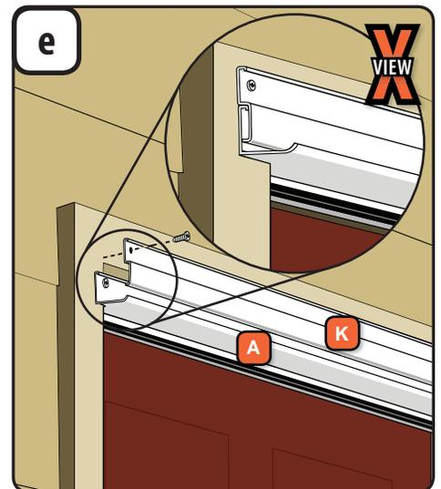
1. Using the drill bit and 1" painted screws from the yellow bag, fasten the rain cap to the mounting surface.
