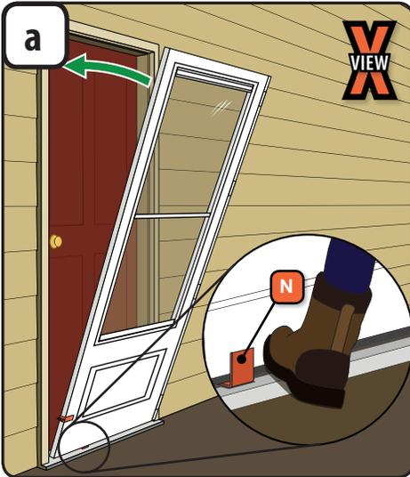
1. Set the door frame on the entry sill so the hinge rail is tight against the mounting surface (or hinge rail shim) and the sill spacer clip is sitting on the door sill.
