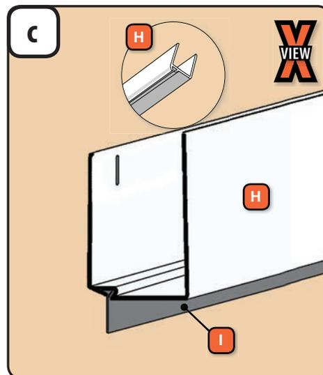
1. **Sweep H only:** Slide the sweep fin (I) into the track in the sweep. Crimp both ends of the track to secure the fin. Trim off excess sweep fin material and properly discard.
