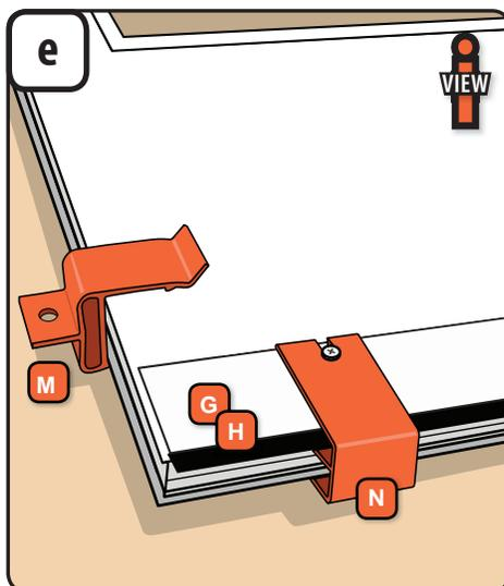
1. Install the sill spacer clip (N) under the latch side sweep screw and tight against the bottom of the sweep (G/H). Tighten the sweep screw to retain the sill spacer clip in place.
