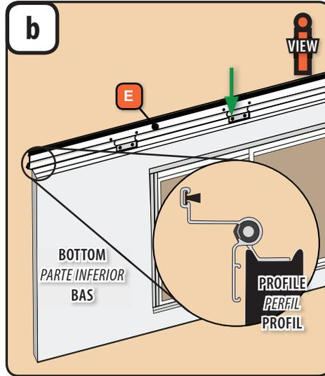
1. Position the hinge rail along the hinge-side edge of the door frame so the bottom hole of the 2nd hinge up from the bottom lines up with the bottom hole from the screw removed in **step 3a**. **NOTE:** The top of the hinge rail should extend approximately 3/16" beyond the top of the door frame.
