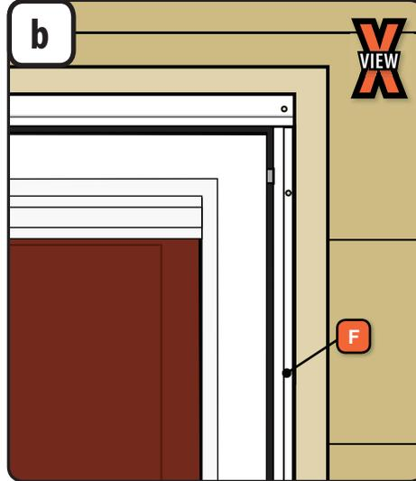
1. Place latch rail (F) in the opening with top end pushed up against rain cap.
