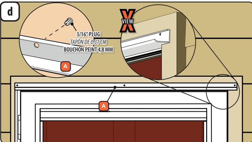
1. Open the storm door. Place the rain cap (A) in the opening so that it rests on top of the hinge rail, aligning the end of the the rain cap with the edge of the hinge rail.
