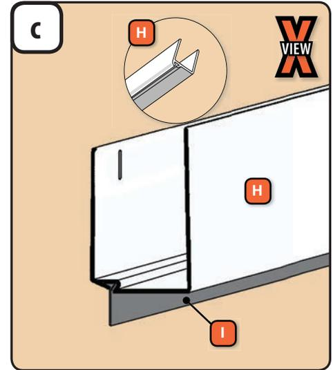
1. **Sweep H only:** Slide the sweep fin (I) into the track in the sweep. Crimp both ends of the track to secure the fin. Trim off excess sweep fin material and properly discard.
