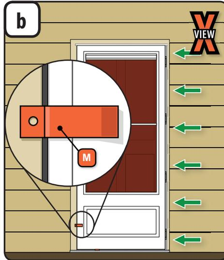
1. The door frame is properly seated in the opening when the hinge rail and latch side spacer clip (M) are flush against the mounting surface and the mounting surface completely fills the hole in the latch side spacer clip. If the latch side spacer clip hole is not completely filled, review **step 2c**.
