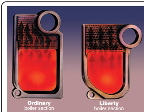
In most boilers, the hot flue gases which rise from the combustion area must pass around the push nipples that join the heating sections. This results in uneven heat transfer, concentrations of soot buildup and undesirable draft loss. Liberty's push nipples are located to the side, out of the way of the flue gases. This creates more uniform heat transfer, minimizes draft loss and reduces soot build-up.
