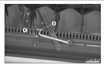
5. Slide lever down between hopper and spike assembly and install other end of shutter link (D) into shutter arm (E).
