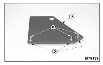
3. Install three transport lock pins (B) into lift plate (C) as shown and fasten with three 5/16 in. lockwashers and hex nuts (D).
