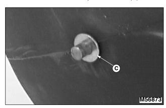
2. Remove the vinyl caps that are over ends of roller assembly axle and slide a 5/8 in. flat washer (C) onto each end.
