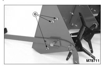
4. Install three transport pins (G) with threaded end to the inside. Secure with 5/16 in. lockwashers and 5/16 in. hex nuts on the inside. Tighten nuts completely.
