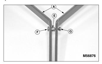
2. Position spacer (E) between frame extension bars (A),
