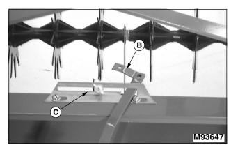
3. Install "L"-shaped end (B) of flow control lever into slot of calibration plate (C).
