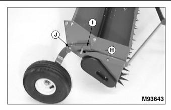
10.Install 3/8 x 2 in. special bolt (H), head of bolt to the inside, into right wheel assembly bracket (I).
