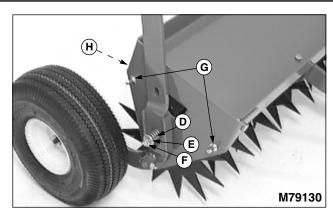
4. Turn tray upright and install two 5/16 in. transport lock pins (G), extending pin to the outside, and fasten with 5/16 in. lockwashers, and 5/16 in. hex nuts (H) to the inside. Tighten nuts.
