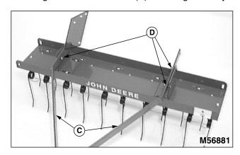
2. Attach tow bars (C) to the inside surfaces of the mounting brackets using three 5/16 x 1 in. carriage bolts and locknuts (D). Hand tighten only.
