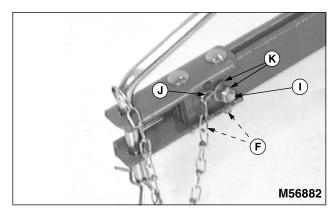
6. Install 5/16 x 1-1/2 in. cross hex bolt (I). Place chain hook (J) around bolt and secure with 5/16 in. flat washer
