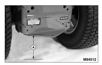
1. Measure length (A) from ground to top of hitch plate with tractor parked on a level surface.
