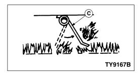
• In position (C), tines are released and flipping thatch upward.
