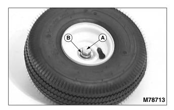
1. Install  $1/2 \times 3 \cdot 3/4$  in. hex bolt (A) and  $17/32 \times 1/16 \times 3/32$  in. flat washer (B) on valve stem side of wheel hub.
