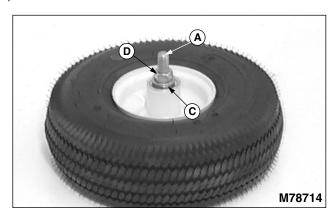
2. Turn wheel over to install second 1/2 in. flat washer (C)
