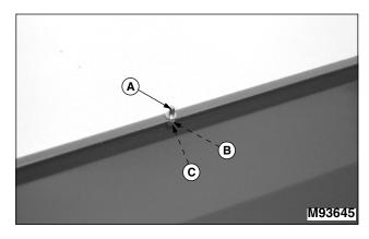
1. Install last transport lock pin (A) into center hole of rear hopper lip and fasten with 5/16 in. lockwasher (B) and hex nut (C).
