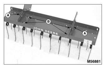
1. Using second set of holes on left side of tray and third set of holes on right side of tray, fasten two mounting brackets (A) to the tine tray with the small flange resting on the tray surface and facing inward. Secure with four 5/16 x 1 in. carriage bolts and hex nuts (B). Hand tighten only.
