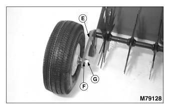
4. Install wheel assembly on lift arm (E), one on each side, and secure with 1/2 in. lockwasher (F) and 1/2 in. hex nut (G). Tighten nut securely so wheel hubs are free to turn on bearings.
