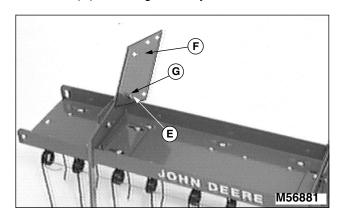
3. Align hole (E) in the lift lock plate (F) with holes in the right tow bar and mounting bracket. Attach the lift lock plate to the inside of the tow bar with a 5/16 x 1-1/4 in. carriage bolt and locknut (G). Hand tighten only.
