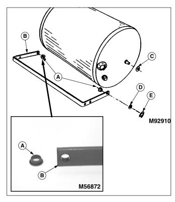
1. Insert a 5/8 in. nylon bearing (A), from inside out, into round hole at each end of scraper frame bar (B).
