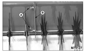
1. Stand tray assembly on its back. Loosen nylock nuts (A) on mounting brackets (B) to ensure proper bracket alignment while installing tow bars.
