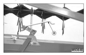
4. Install one end of shutter link (D) into end of flow control lever.
