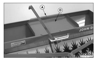
2. Install weight tray (D) over pin (A) and hopper lips as shown.
