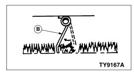
In position (B), tines are under tension and working.
