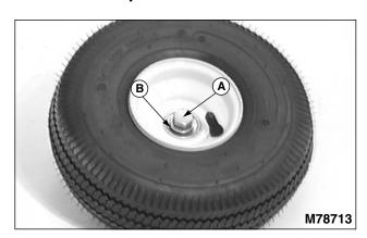
1. Install 1/2 x 3-3/4 in. hex bolt (A) and 1/2 in. flat washer (B) on valve stem side of wheel hub.
