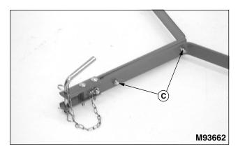
9. Tighten tow bar nylock nuts (C).
