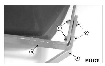
1. Attach short end of each frame extension bar (A) to scraper frame bar (B) and fasten with two  $5/16 \times 1$  in. hex bolts (C) and two 5/16-18 in. nylock nuts (D) on each side. Frame extension bars will meet at center. Hand tighten only.
