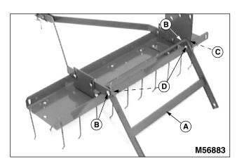
1. Attach carriage frame assembly (A) (side with two holes should be next to lift lock plate) to rear holes (B) in tow bars and lift lock plate at right side (C). Secure with  $3/8 \times 1-1/4$  in. hex bolt (left side) and  $3/8 \times 1-1/2$  in. (right side lift lock plate), 3/8 in. bushings, 3/8 in. flat washers, and fasten with 3/8 in. locknuts (D). Tighten so bar is secure but free to pivot.
