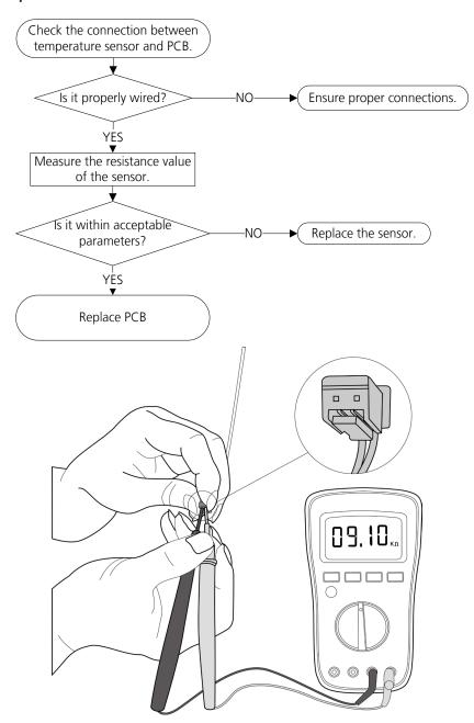
Note: For certain models, outdoor PCB could not be removed separately. In this case, the outdoor electric control box should be replaced as a whole. This picture and the value are only for reference, actual appearance and value may vary
