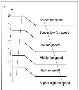
To meet T4>T4HeatLimit\_ADD\_3, first determine the initial fan based on T4. After the initial fan runs for 30s, correct the outdoor fan based on the average temperature of T2 (when the temperature enters the critical point, it takes 10s to reach the critical point to be effective). Select a lower gear for the first gear or (super) breeze speed.
