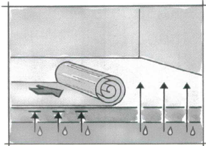
**Underlayment must be used under engineered floors**
