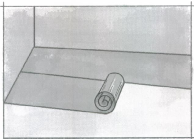
**Roll underlayment out carefully overlapping each new edge, and securing the adhesive**
