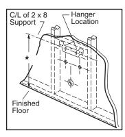
Determine the desired rim height (for example 32") then select from the Table at right the height of the hanger mounting bolts centerline
