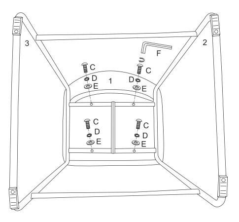
Attach the seating frame (1) to the metal frame (2)(3) and secure it by using washers (E), spring washers (D) and wrench (F).
