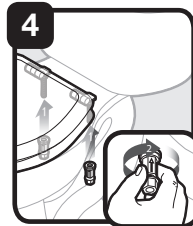
Attach nuts, Finger-tighten
