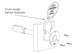
Tip: Drilling into brick or stone? Consider using specialized fasteners and/or anchors. We also manufacture optional stainless steel mounting plates to space the mounting holes out further if needed.
