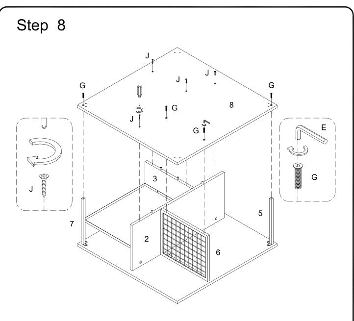
Using bolt (G) attach part (8) into parts (5,6,7) with hex key (E), then using screw (J) attach part (8) into parts (2,3) with Philips head screwdriver as per diagram.
