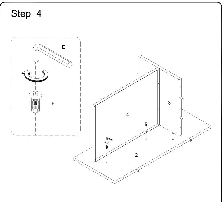
Attach part (3) to part (2) and using bolt (F) secure part (4) into part (2) with hex key (E) as per diagram .
