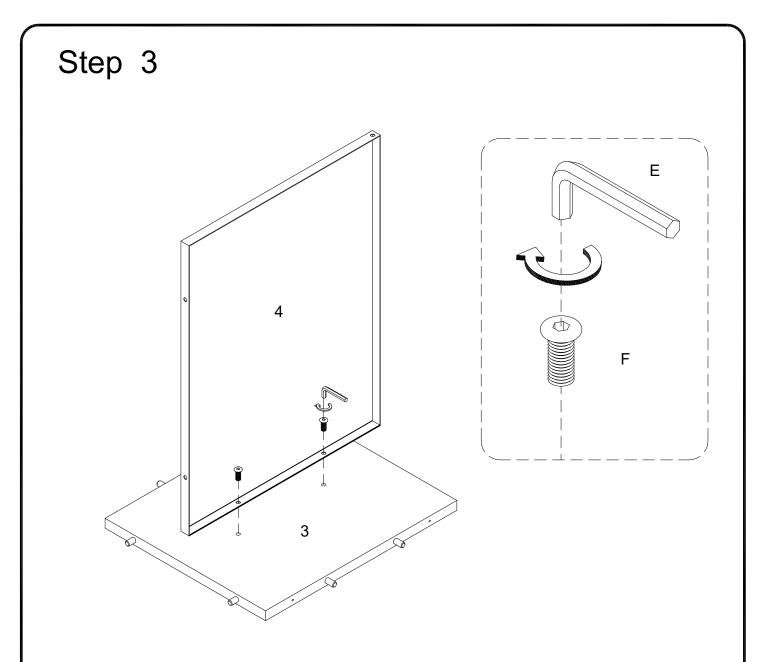
Using bolt (F) attach part (4) into part (3) with hex key (E) as per diagram. Note: Do not tighten all bolts .
