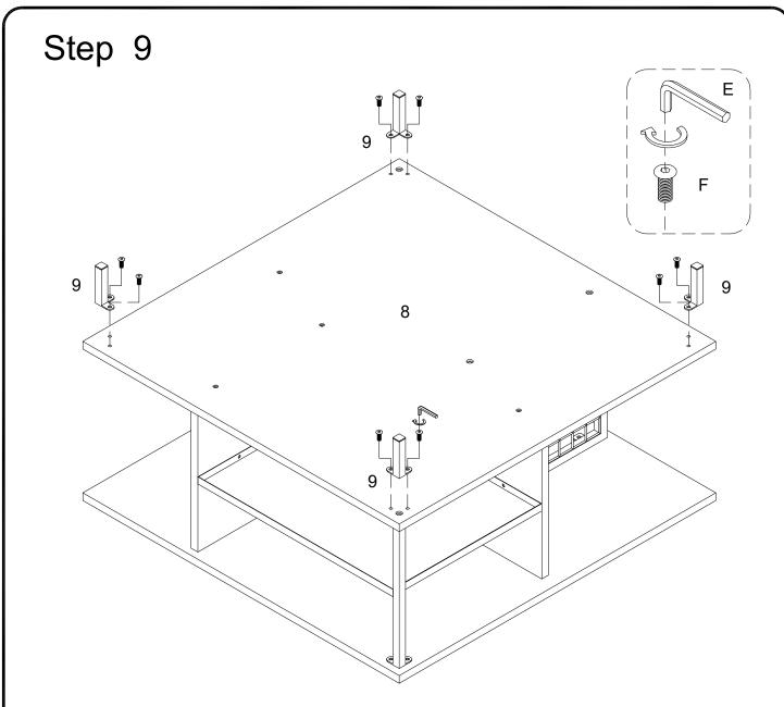
Using bolt (F) attach part (9) into part (8) with hex key (E) as per diagram. Note: tighten all bolts .
