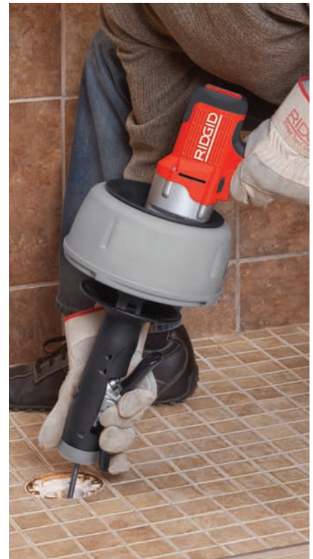
The ¾" cable in Model K-45AF-5 and K-45AF-7 extends machine's capacity to 2½" drain lines.
