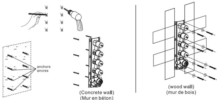
1. Make marks according to the size of the main body valve, and then drill anchors into the wall (concrete wall).
