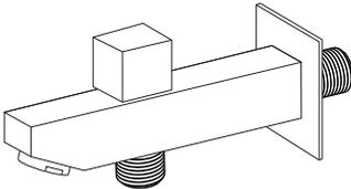
Install the decorative cover under the water spout, and then tighten it into the wall using the waterproof tape.
