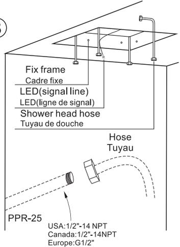
Connect one end of the corrugated pipe to the embedded PPR water pipe and the other end to the water inlet pipe on the back of shower head.
