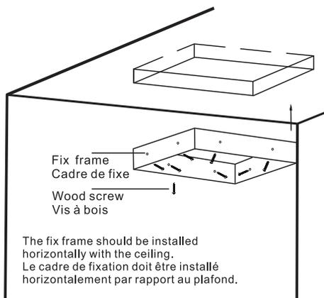
Fasten the fix frame to the wooden frame with screws
