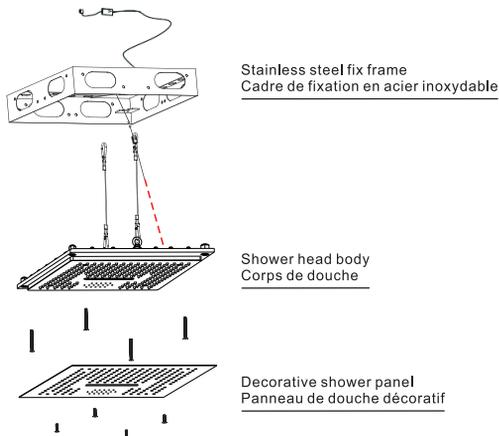
According to the mark (Remove/Install) on the top of the shower head panel, unscrew the decorative shower panel, shower head body, and fix frame respectively.
