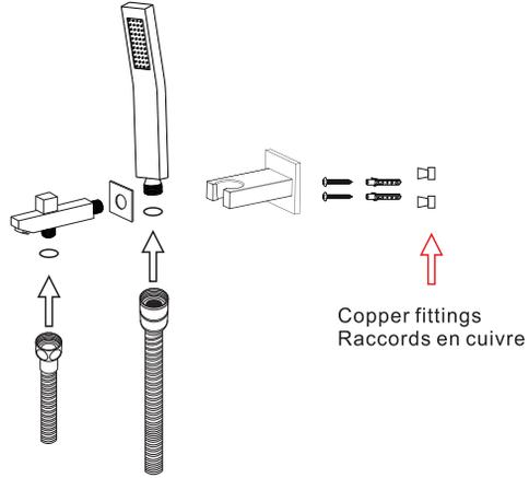
Step 1. First, use anchors to screw the pipe holder into the wall.
