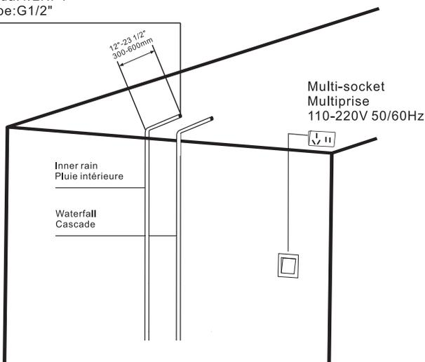
Install the power switch in the appropriate position, lay out the water pipeline, and connect it to the main body.
