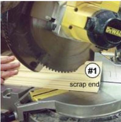
Sometimes it may be necessary to splice crown mouldings together on a long wall.
