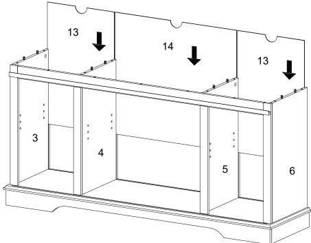
Slide back panel (13,14) into grooves as per diagram.
