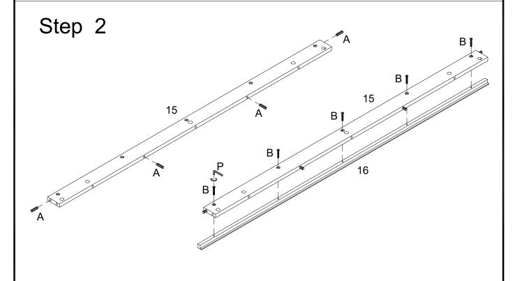
Insert wooden dowel (A) into part (15). Attach part (15) to part (16) using bolt (B) with hex key (P).
