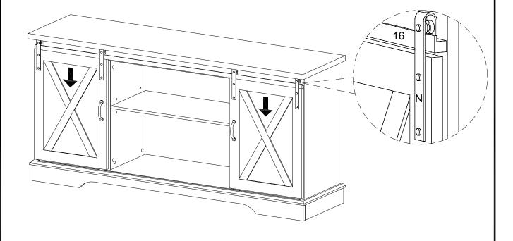
Hang pulley (N) to part (16), then press down to hold the door.
