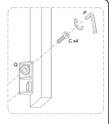
Attach connector (Q) to part (2) using bolt (C) with hex key (P).
