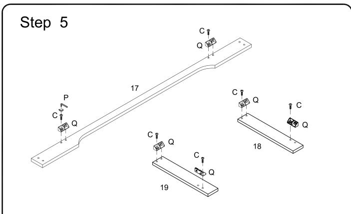
Attach connector (Q) to part (17,18,19) using bolt (C) with hex key (P).
