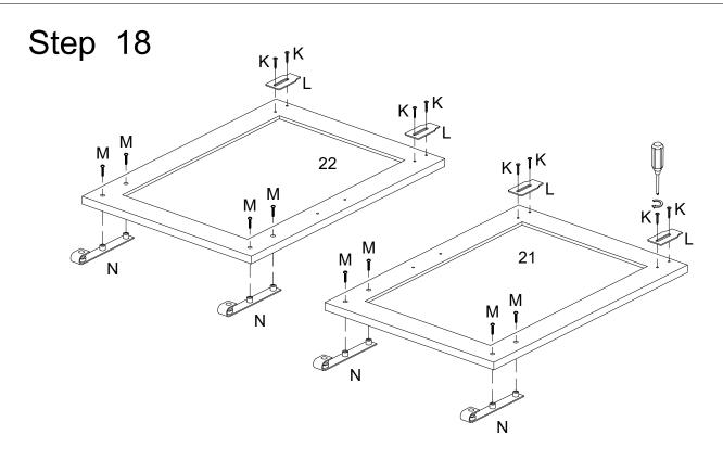
Attach pulley (N) using bolt (M), and plate (L) using screw (K) to part (21,22) with screwdriver.
