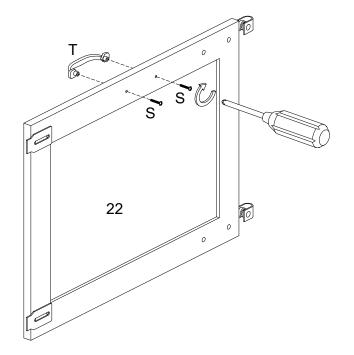
Attach handle (T) to part (21,22) using bolt (S) with screwdriver.
