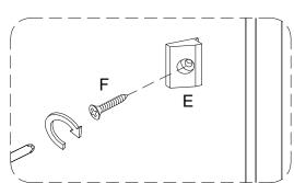
Attach plastic wedge (E) to part (13,14) using screw (F) with screwdriver.
