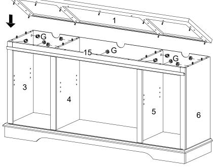
Attach part (1) to part (3,4,5,6), then insert and secure cam lock (G) to part (3,4,5,6) to lock it.
