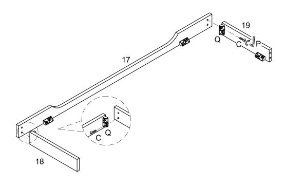
Attach connector (Q) to part (17) using bolt (C) with hex key (P).
