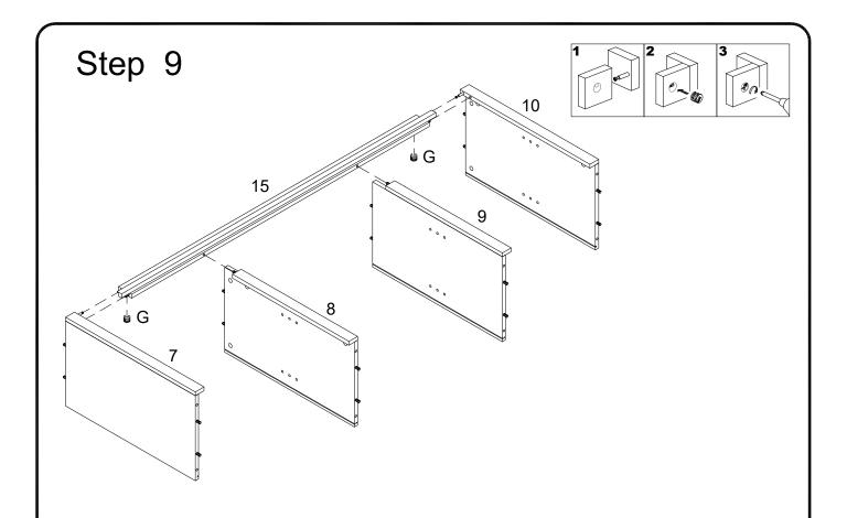
Attach part (7,8,9,10) to part (15), then insert and secure cam lock (G) to part (15) to lock it.
