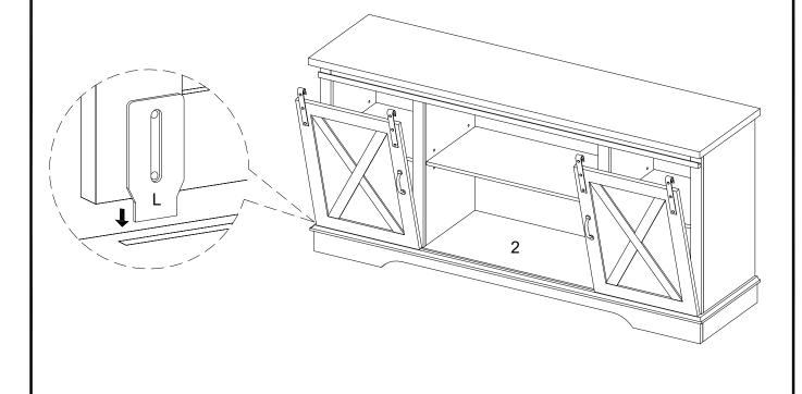
Place plate (L) on door into groove.
