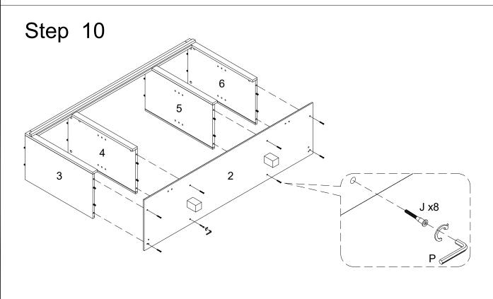
Attach part (2) to part (3,4,5,6) using bolt (J) with hex key (P).
