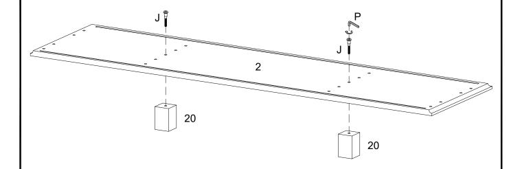
Attach part (20) to part (2) using bolt (J) with hex key (P).
