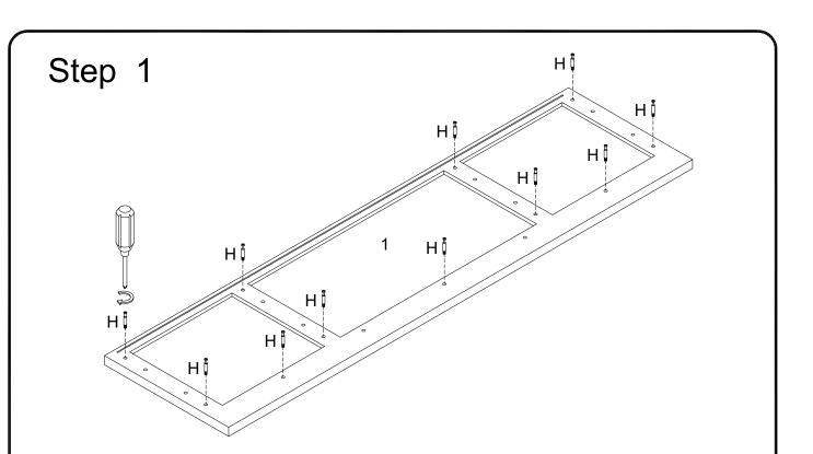
Attach cam bolt (H) to part (1) with screwdriver.
