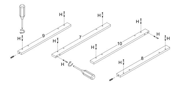
Attach cam bolt (H) to part (7,8,9,10) with screwdriver.
