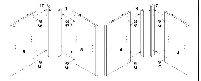
Attach part (7,8,9,10) to part (3,4,5,6), then insert and secure cam lock (G) to part (3,4,5,6) to lock it.
