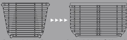
Adjust-A-Grate window well covers are designed to offer you a custom fit without the hefty price. Each loop on the grate moves independently, allowing the grate to adjust side to side to perfectly conform to a variety of well sizes and contours within the given range. Ensure you select the correct model for your well opening's size and shape.
