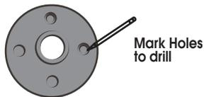
3. Pre-drill 3/16" holes at each mark you will be using anchors. Do not pre-drill if you are screwing into a stud.
