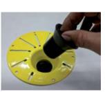
4. Apply glue to the outside of the ABS or PVC 1 ½" pipe and to the inside of the P-trap.
