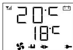
Power on status (automatic mode)
