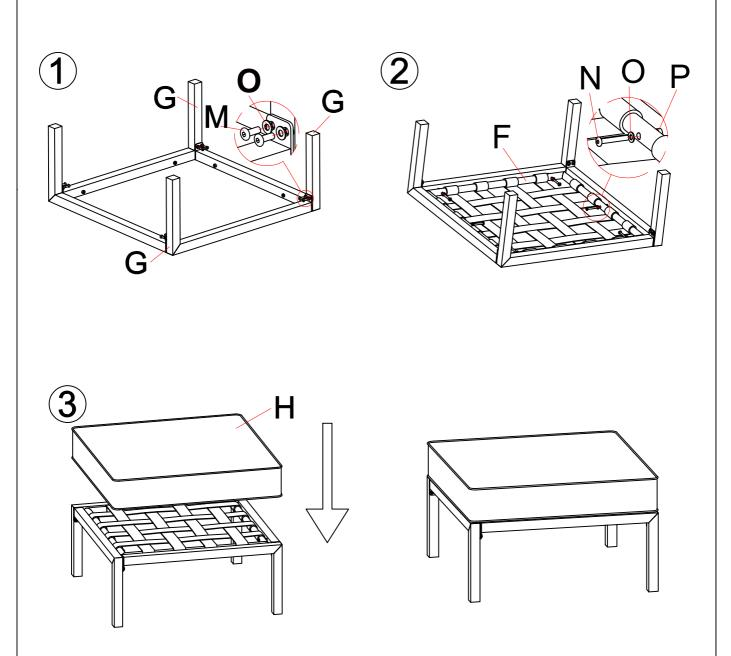
In order to facilitate the assembly and make your final product firm and stable, please tighten by a few rounds each screw one by one. After all screws are connected, then you start to tighten each screw to the end. DO NOT tighten any screw to the end before you've connected all screws.
