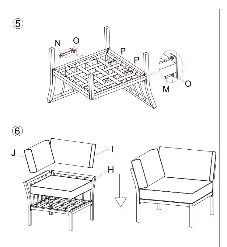
In order to facilitate the assembly and make your final product firm and stable, please tighten by a few rounds each screw one by one. After all screws are connected, then you start to tighten each screw to the end. DO NOT tighten any screw to the end before you've connected all screws.
