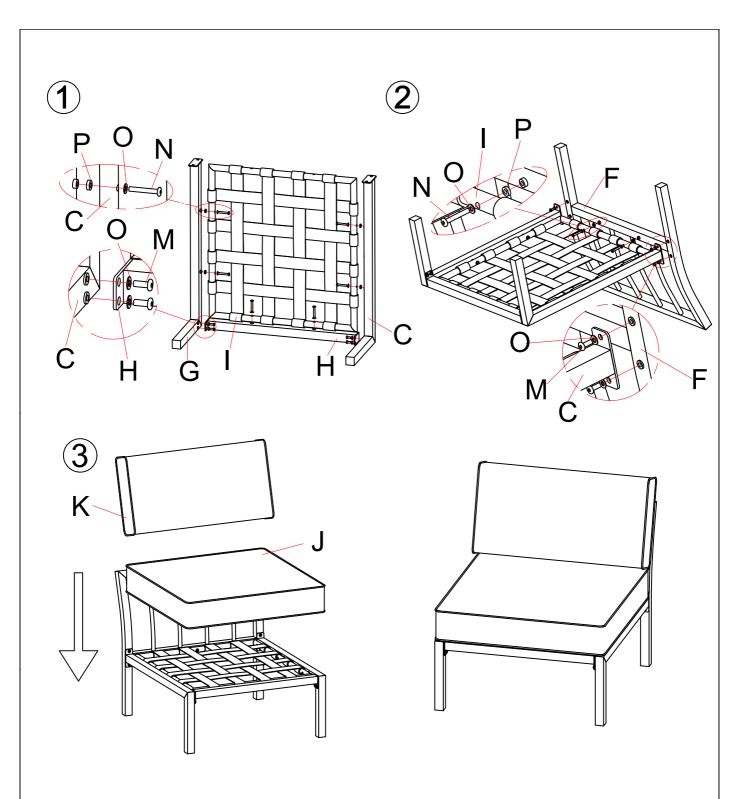
In order to facilitate the assembly and make your final product firm and stable, please tighten by a few rounds each screw one by one. After all screws are connected, then you start to tighten each screw to the end. DO NOT tighten any screw to the end before you've connected all screws.
