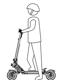
3. Put one foot on the footboard and another foot on the ground. Then, push the scooter forward.
