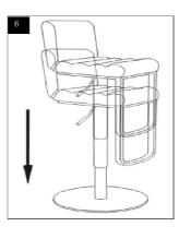
Step 6 The height can be adjusted by holding the handle underneath the seat.
