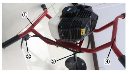
2.Set the auger on the output shaft, insert the type D pin, then lock it .
