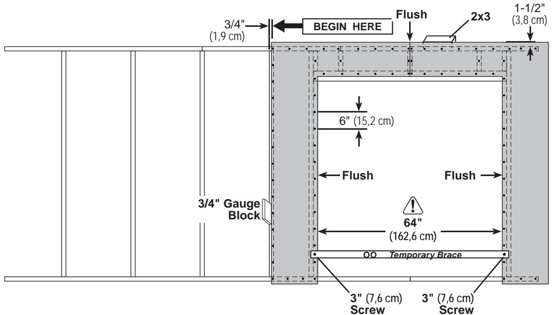
Secure panels with 2" nails spaced 6" apart on edges.
