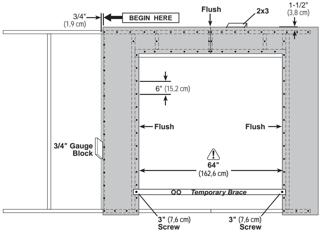
**5** Install (1) 48" x 84" panel flush to installed panels and 1-1/2" from the top plate.
