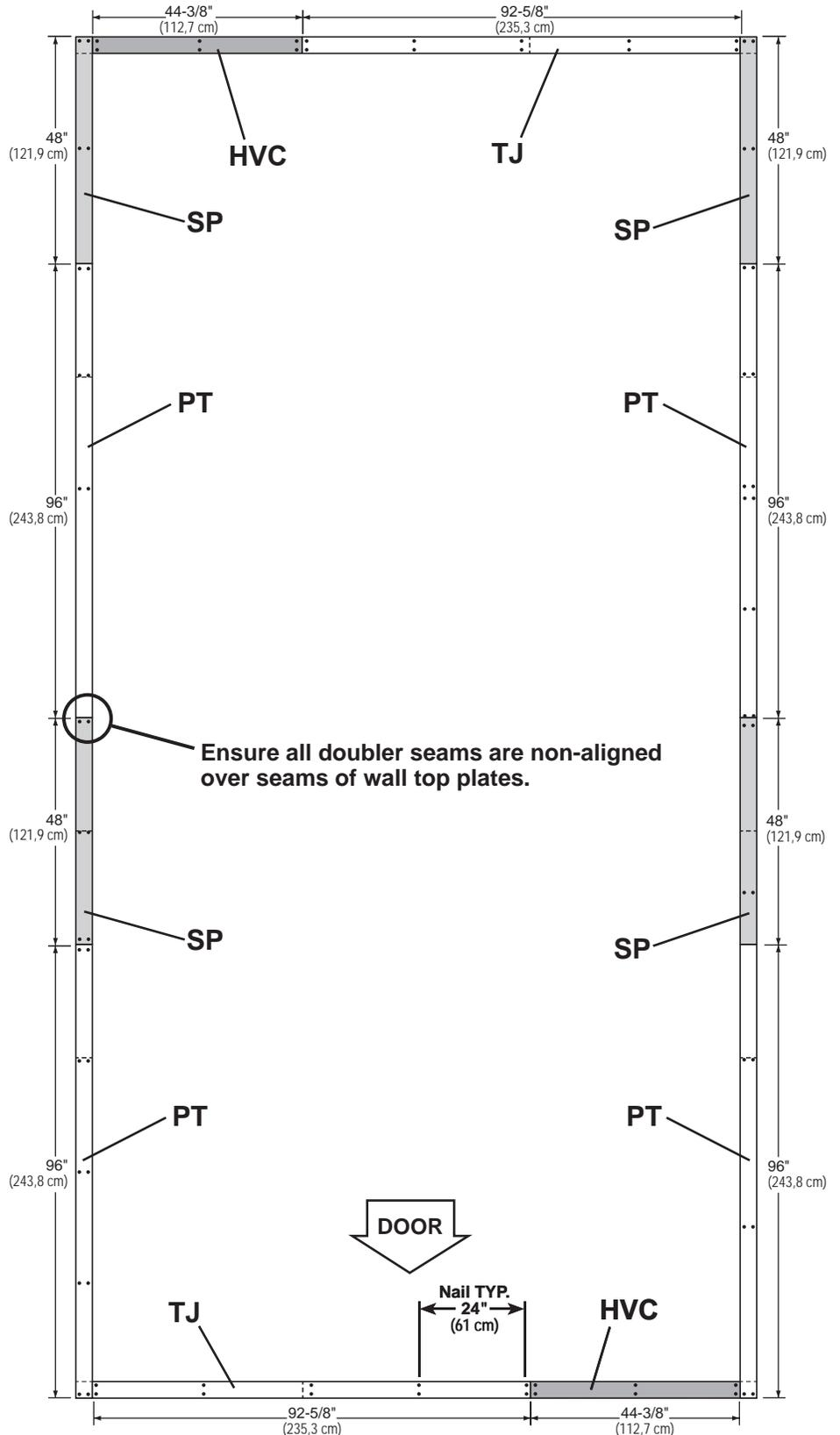
Ensure all doubler seams are non-aligned over seams of wall top plates.
