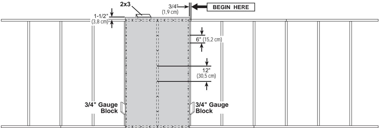
**3** Install (5) 48" x 84" panels flush to installed panels. Locate panels 1-1/2" from the top plate.
