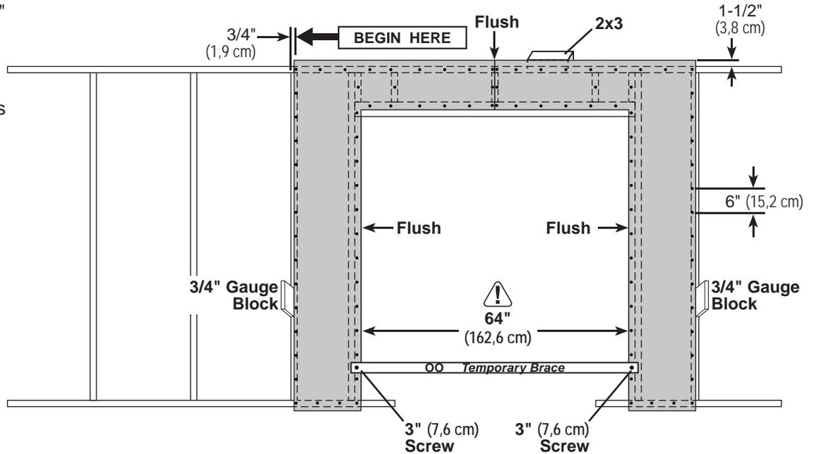
Secure panels with 2" nails spaced 6" apart on edges.
