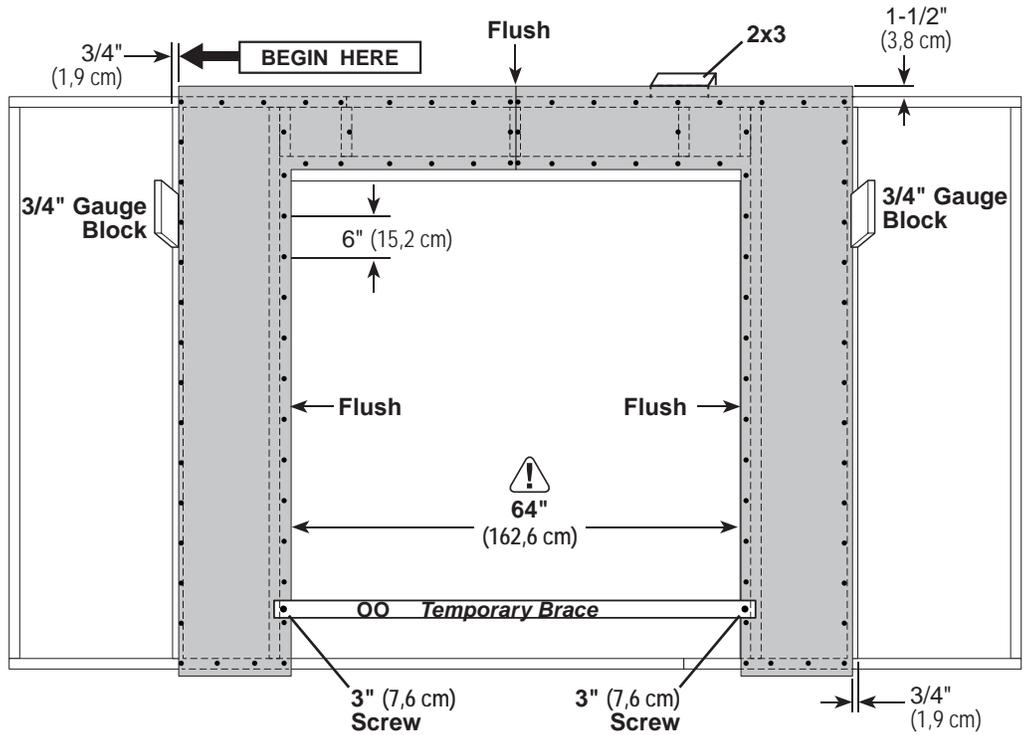
**5** Install (2) 11-7/8" x 84" panels flush to installed panels and 1-1/2" from the top plate.
