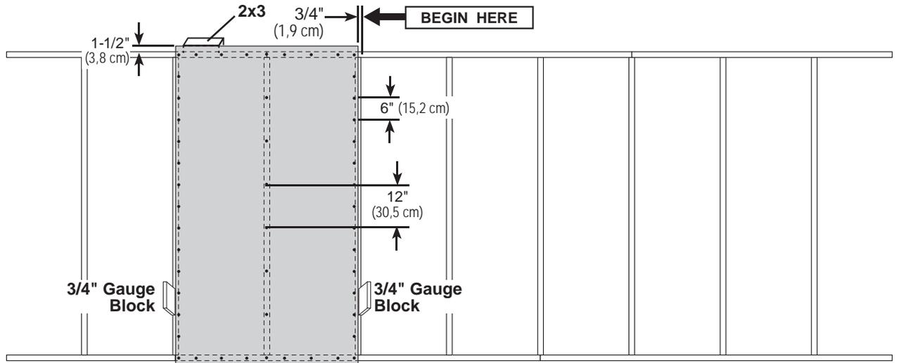
**3** Install (4) 48" x 84" panels flush to installed panels. Locate panels 1-1/2" from the top plate.
