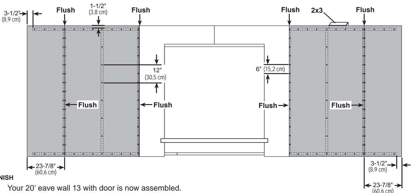
Your 20' eave wall 13 with door is now assembled. Carefully flip the wall over.
