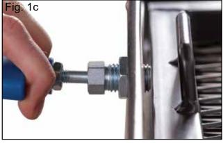
**Step 2.** Flip the carrier basket upside down and slide the hitch tube assembly into the center support tube. Install the leveler bolts (J) and nuts (K). These will be adjusted later. Align the holes and insert a pin with clip (E). Install two bolts (H) with nuts (I) and tighten until seated using a 7/8" wrench. Do not over-tighten.
