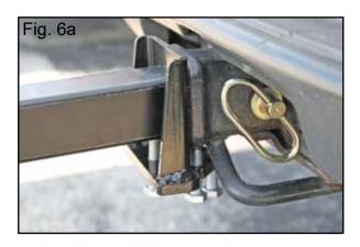
Step 6b. Pinch Bolt - 2nd Option: Insert the carrier into the hitch and install the pinch bolt assembly.
