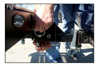
Remove the pin with clip (E) to fold the carrier vertically. Replace the pin in the top pin hole to secure the carrier in the vertical position.
