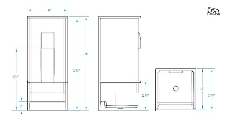
FEATURES | Ibs | Dimensional Tolerance ± %". Dimensions needed for site preparation should be measured from the unit. Aquatic assumes no responsibility for preparatory work.
