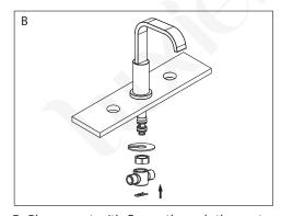
B. Place spout with flange through the center mounting hole on the mounting surface. Secure spout with metal washer and metal nut. Once the spout is secured. Push the T connector onto the mounting tube until it snap into place. (Caution: The 2 rubber o-rings must be seated properly in the grooves on the mounting tube.) Lock the T connector in place by firmly inserting the locking pin.
