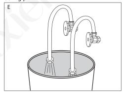
E. It is highly recommended to flush the water lines before connecting the water supply hoses (not included) to the faucet. Place a water bucket under the cabinet, with both water supply hoses inside the bucket. Slowly turn on the valves and let water run for about 45 seconds.
