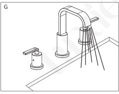
G. Turn on water supply and allow the unit to run for about 1 minute while check for leaks at all connections.
