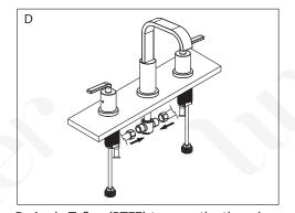
D. Apply Teflon (PTFE) tape on the thread of the T connector and connect the water inlet hoses to the T connector. Use an adjustable wrench to tighten the fittings. Do not overtighten the connection. (IMPORTANT: The black hoses are longer by design to accommodate wider installation. For narrower installation, it is strongly recommended to loop the hoses around before connecting to the T connector to avoid any kinks. Turn the T connector at an angle will make connecting the black hoses
