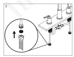
F. Apply Teflon (PTFE) tape on the thread in a counter-clockwise direction.
