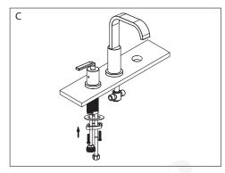
C. Slide hot and cold water handle / valve through mounting holes. Make sure the connecting hoses are installed toward the center spout. Handles should point outward in off position. Secure the handles with metal washers and mounting nut. Hand tighten the nut onto the valve and secure it by tightening the screws
