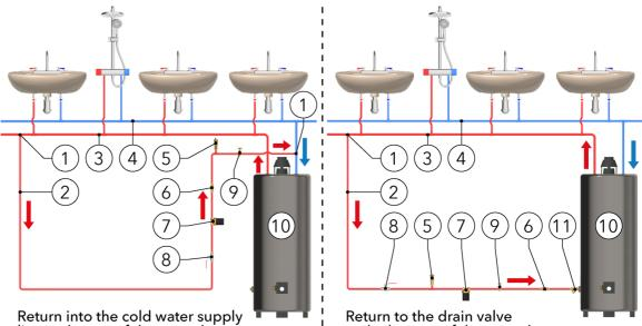
Return into the cold water supply line at the top of the water heater
