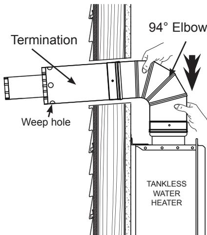
The weep holes around the outside of the termination must be at least 1 inch from the finished wall of the building. See Figure 4.
