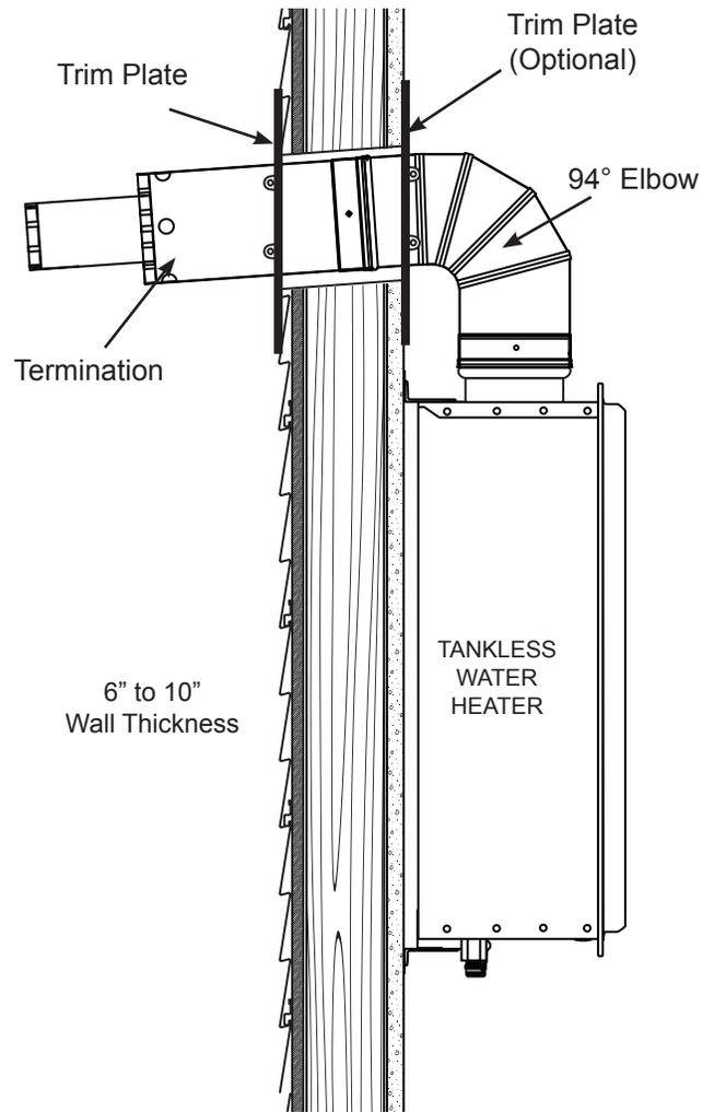
This kit can be extended up to the maximum allowable lengths as listed in the Use and Care Manual provided with the water heater. **NOTICE:** If a vent length of more than two (2) feet straight up from the top of the water heater is needed, a condensate collector must be installed at the water heater.
