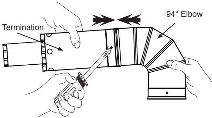
**Horizontal Termination and Elbow Installation** - Align the elbow and termination vent assembly through the hole in the wall. Align and press the elbow down onto the appliance adapter. Completely seat and secure the connection per the joint assembly instructions. A slight rotation of the joint may be necessary to line up the venting. The venting should be square and sealed at final assembly.
