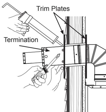
**Clearance Considerations** - The concentric vent piping and fittings are certified for a clearance of zero (0) inches to combustible surfaces.
