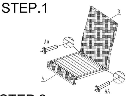
Please connect A and B with AA. The screws have to be screwed in halfway, not to the end.
