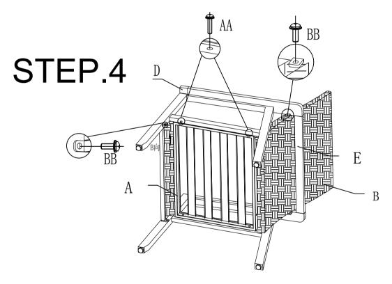
Please insert D into E,and connect D and A&B with AA&BB. When A/B/D/E are ready,tighten AA&BB to the end.
