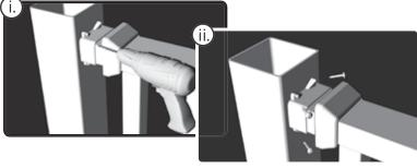
For angled rail installation other than at  $90^\circ$  or  $180^\circ$  purchase left to right angle brackets.
