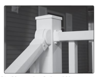
Note: Select Stair Railing sections will rack to a maximum of 32 degrees. If your custom installation calls for a greater angle you will need to route the hole openings to a longer length.
