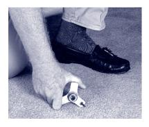
Place the screw gripper, on the alignment fixture, over the screw head. Then rock the fixture left to right snapping the head off. The screw breaks at the weak spot that is consistently set below the surface of the floor. Squeaks are gone and no damage is done the carpet.
