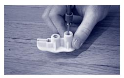
After pre-drilling a <sup>1</sup>/<sub>8</sub> inch hole down 2 <sup>1</sup>/<sub>4</sub> inches, drive a screw through the taller opening in the fixture.
