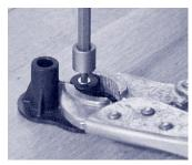
ers, like Vise Grips<sup>®</sup>. By lifting up on the pliers and slowly reversing the drill, the screw will come back out.
