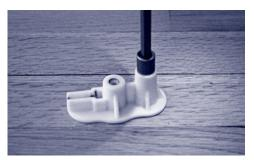
Drive the screw down as far as the fixture will allow.
