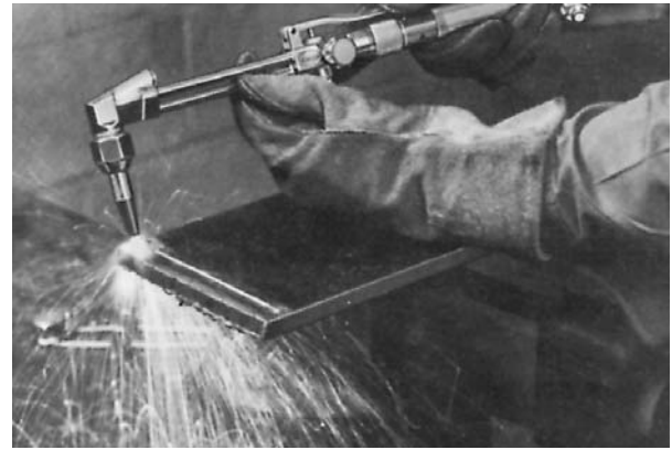
Figure 19. Steel Flame Cutting
