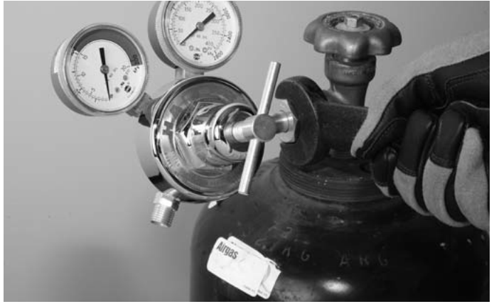
Figure 3. Attaching Fuel Gas Regulator
