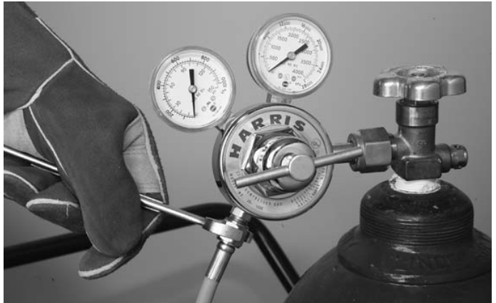
Figure 4. Attaching Hose to Regulator
