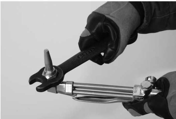
Figure 7. Installing Cutting Tip
