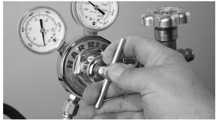
Figure 8. Regulator Adjusting Key
