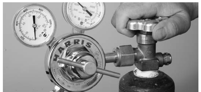
Figure 10. Opening Oxygen valve
