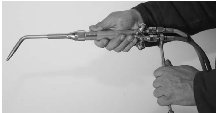
Figure 5. Attaching Hose to Torch
