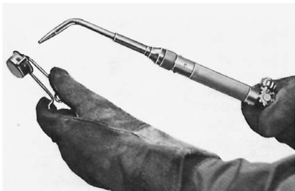
Figure 11. Igniting Fuel Gas
