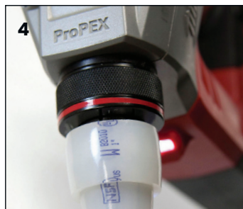
Figure 13: Expansion with Milwaukee M18 ProPEX Expansion Tool
