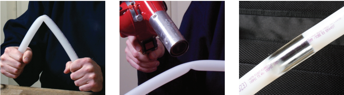
Figure 5: Reforming Kinked Piping
