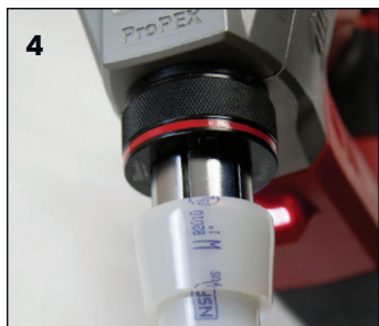
Figure 13: Expansion with Milwaukee M18 ProPEX Expansion Tool
