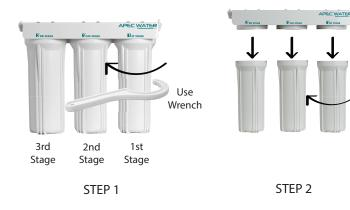
After taking the housing off, take out the dirty filters and put the 3 new filters in. Remember, Stage 2 and Stage 3 are the same carbon filters.
