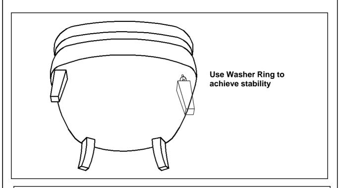
Install the B1 leg into the chair front by putting a Washer Ring (optional) on the threaded stem and then insert the threaded stem into the threaded hole at the corner of the bottom of the chair. Tighten by turning leg clockwise. Repeat the same procedure to install the other 3 remaining legs.
