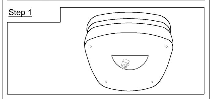
Position the Chair on tis back, as shown. Unzip to open and remove the 4 wooden legs. Close the pouch.
