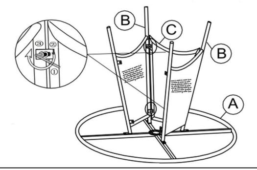
Attach Leg Support Panel(C) between Leg Panels(B) using Bolt(③) and Washer(②) with Allen Key(①) as shown in the picture above.
