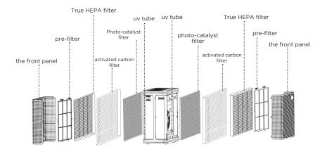
The FILTER REPLACEMENT indicator light will be slowly flashing red after 2160 hours of use. The HEPA and CARBON filters should be replaced at the same time. You may need to replace them sooner if you are using the air purifier in an environment with poor air quality. If you notice that the filters do not appear visibly clean, or air purification seems to have decreased, the filters should be replaced.
