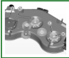
GXT002378-UN: Remove Sheave
