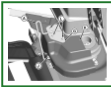
GXT002377-UN: Install Front Blower Belt Shield
