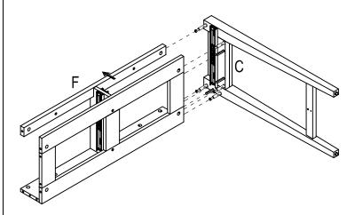
d) Tighten bolt (BB) with lock (CC) in the pre-drilled holes.
