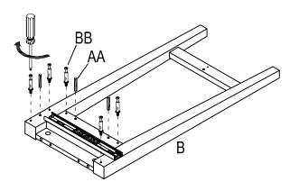
□ c) Join frame (B) and bar (H) to the assembled body with dowel (AA).
