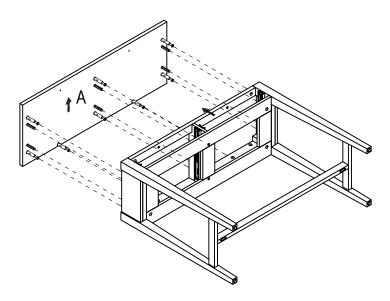
d) Tighten bolt (BB) with lock (CC) in the pre-drilled holes. Tighten bar (F) with screw (DD).
