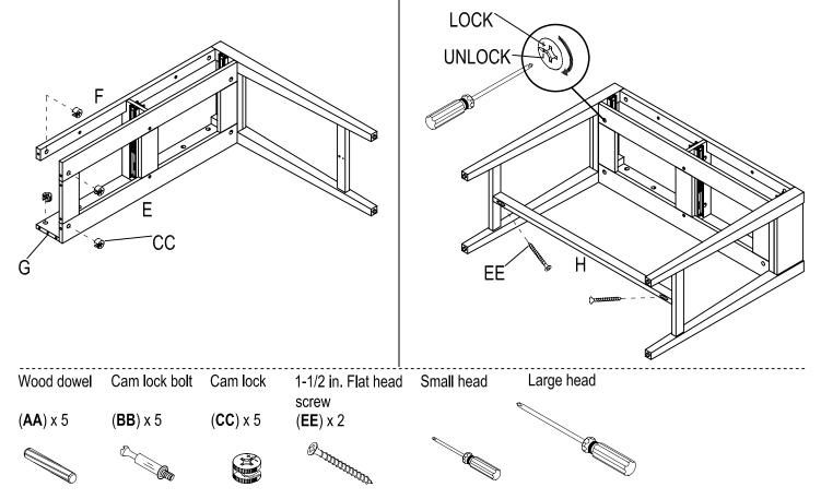
$\hfill\square$  b) Insert lock (CC) into panels (E) and (G), bar (F).
