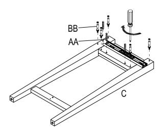
c) Join frame (C) and bar (F) to the assembled body with dowel (AA).
