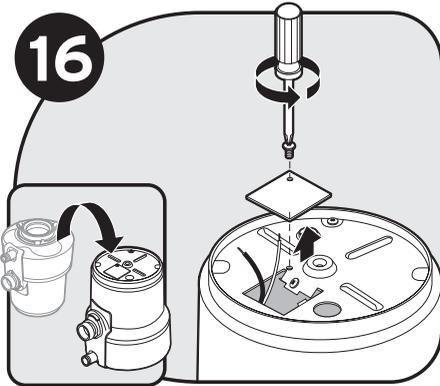
Turn disposer over and remove electrical cover plate. Pull out wires.
