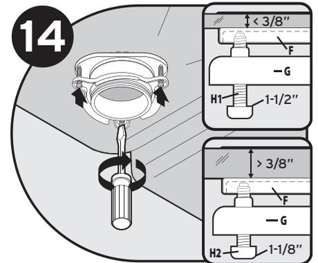
Tighten 1-1/2" screws (H1) evenly and firmly against backup flange. Use shorter 1-1/8" screws (H2) if sink is more than 3/8" thick.
