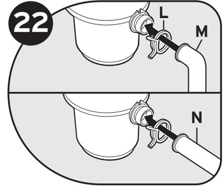
Place tube (M or N) into Anti-Vibration Tailpipe Mount™. Use provided tubes for best results. Secure with spring load hose clamp (L) (provided).
