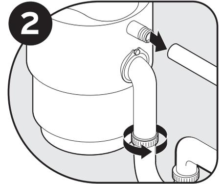
Turn off electric power at circuit breaker or fuse box. Disconnect drain trap from waste discharge tube. Disconnect dishwasher if connected to the disposer.
