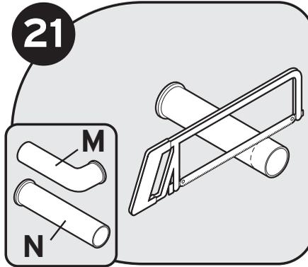
You may need to trim discharge tube (M or N) to ensure proper fit.
