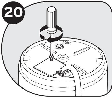
Push wires into disposer and replace electrical cover plate.
