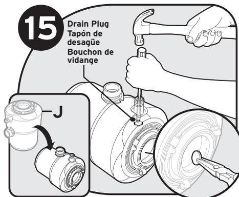
**NOTICE:** Drain plug cannot be replaced once it is knocked out. Turn disposer (J) onto side and knock out drain plug with screwdriver. Remove plug from inside of disposer with pliers.
