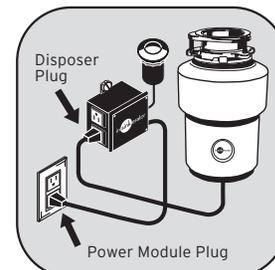
• Plug power module cord into a dedicated, grounded 120V AC outlet that is continuously energized.
