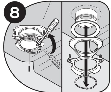
Using a screwdriver, remove the snap ring (I).
