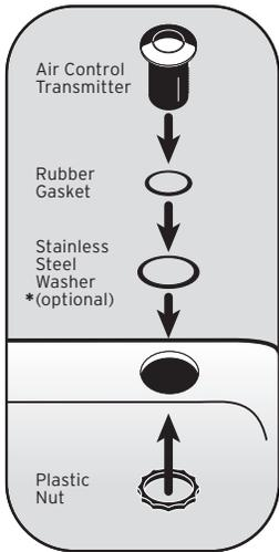
• Mount the push button directly through a standard sink hole.
