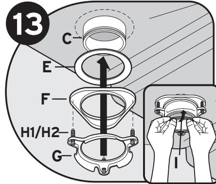
Insert fiber gasket (E), backup flange (F) and mounting ring (G). Hold in place while inserting snap ring (I). Pull snap ring (I) open and press firmly until it snaps into place.
