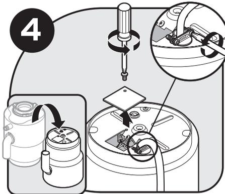
Flip disposer over and remove electrical cover plate. Save cable connector if applicable.
