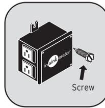
• Mount power module on a cabinet wall within 3 feet of an electrical outlet and the disposer.
