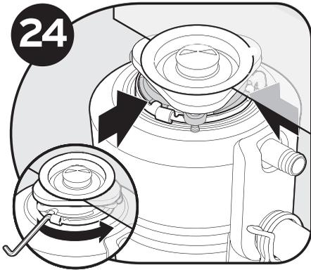
Turn mounting ring until all 3 mounting tabs latch over the ridges on the slide-up ramps.
