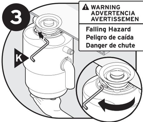
Support disposer, insert end of wrench (K) into right side of mounting lug, and turn. Disposer will fall free.
