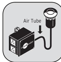
• Attach air tubing between push button and power module.
