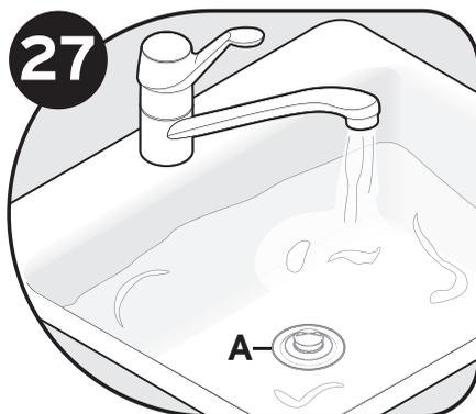
Insert stopper (A) into sink opening. Fill sink with water, then test for leaks. Reconnect electrical power at fuse box or circuit breaker box.
