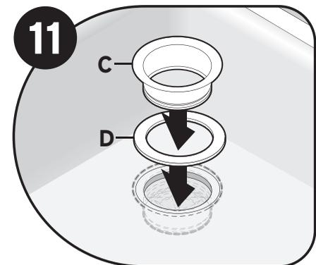
Working from the top of the sink, place rubber gasket (D) under sink flange (C). Ensure sink hole area is clear of debris and place sink flange/gasket into sink hole.
