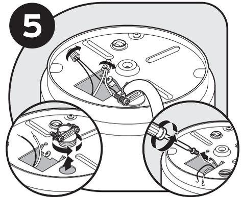
Disconnect the disposer wires from the electrical supply.
