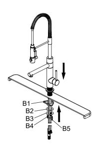
Insert faucet through hole in sink or countertop.From underneath sink, attach the seat (B1), rubber washer (B2), metal washer (B3), and nut (B4). Lock nut (B4) into position by tightening screws (B5).
