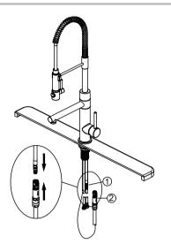
Push the quick connector (2) firmly upward and attach it to the receiving block (1). Pull down moderately to ensure the connection has been made.
