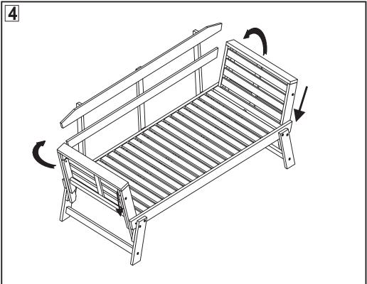
Step 3: attach the back (A) to the seat (B) as shown on the picture. Then use the Allen bolt L (G1) and the Allen bolt S (G2) in the middle, left and right use Allen bolt M ( G8) and tighten by the Allen Key (G7) and wrench (G6) as shown on the picture. Make sure put correct position to use the Allen bolt L(G1) , the Allen bolt S (G2) , the Allen bolt (G8) as shown on the picture.
