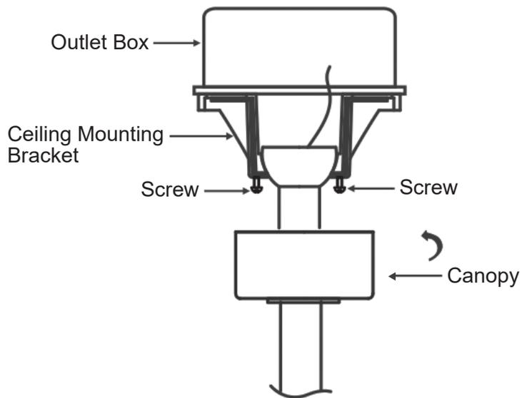
**Step 1.** Tuck all the connections neatly into the ceiling outlet box.
