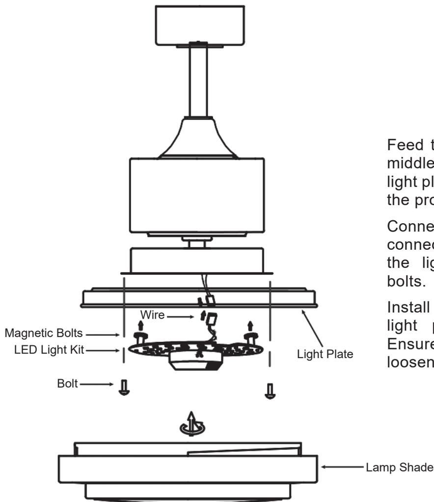
Feed the wire connector through the middle of the light plate. Install the light plate on the motor assembly with the provided bolts.
