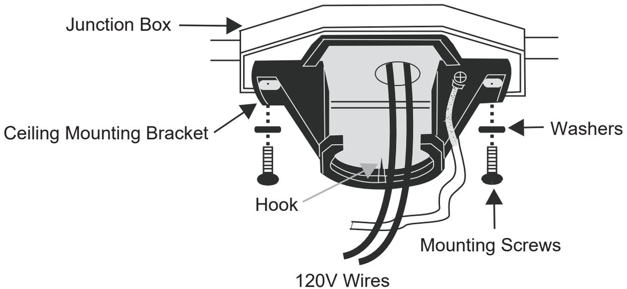
Loosen the 4 screws on the mounting bracket. Use the screws and washers to attach it to your ceiling.
