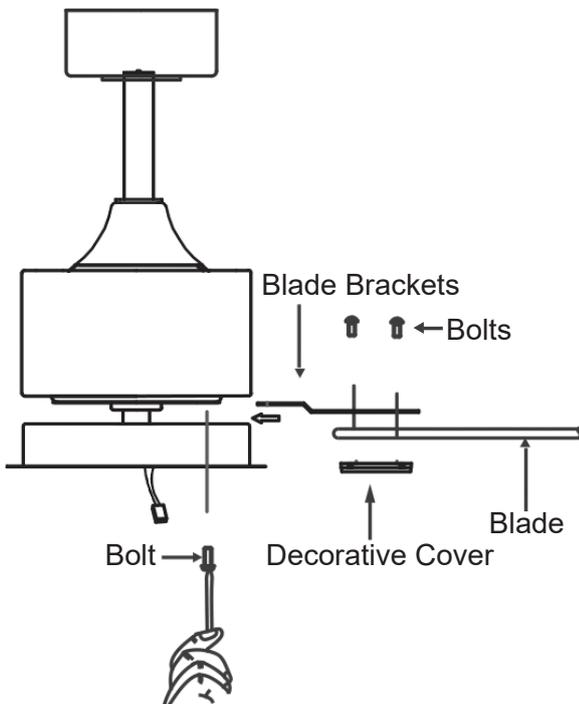
Loosen the bolts & washers pre-installed on blade holder. Insert the blade through the blade slot in the motor housing. Align the holes on blade and blade holder and use the provided washers and bolts to connect them. Repeat this process with the other blades.
