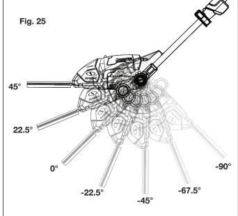
**4.** Rotate the cutting head to the desired cutting angle while pressing the angle adjustment button (Fig. 26).
