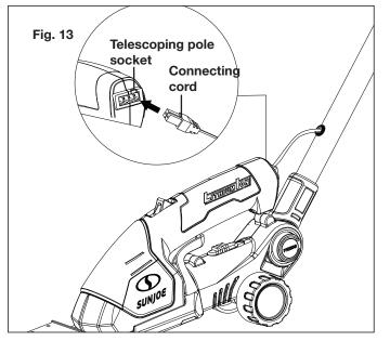
4. To disconnect the grass shear + hedge trimmer from the telescoping pole, unplug the connecting cord from the telescoping pole socket, and remove the grass shear + hedge trimmer from the pole head while pressing the cutting head lock (Fig. 14).
