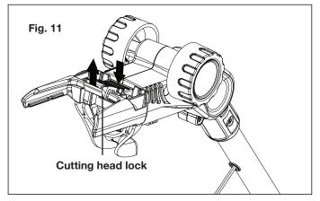
While pressing the cutting head lock, align the grass shear + hedge trimmer with the pole head, and insert the grass shear + hedge trimmer into the opening of the pole head. Release the cutting head lock when the grass shear + hedge trimmer fits into place (Fig. 12).
