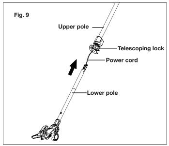
2. When the pole reaches the desired length, latch the telescoping lock by pushing it back down (Fig. 10).
