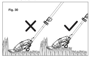
6. Keep the cutting device at an angle of about 10° to the ground when shearing. Avoid touching the ground as this can ruin the lawn and damage the product.
