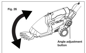
**5.** Release the button when the cutting head is fixed into the desired angle.
