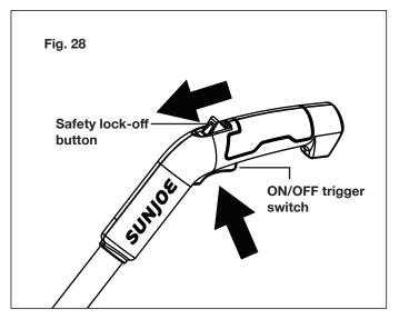
4. To power OFF, simply release the ON/OFF trigger switch.
