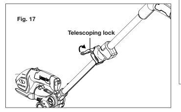
2. Pull the lower pole out or push it together to adjust to the desired length (Fig. 18).
