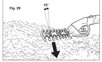
Shaping – A hedge should be trimmed to achieve a trapezoidal form; it should widen toward the bottom on both sides. Shaping a hedge in this manner improves the penetration of light to the lower extremities. A general guideline is to slant the hedge approximately 4 in. (10 cm) for each 39 in. (1 m) of hedge height.
