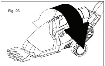
**3.** When the cutting head clips in the desired angle, release the angle lock button.
